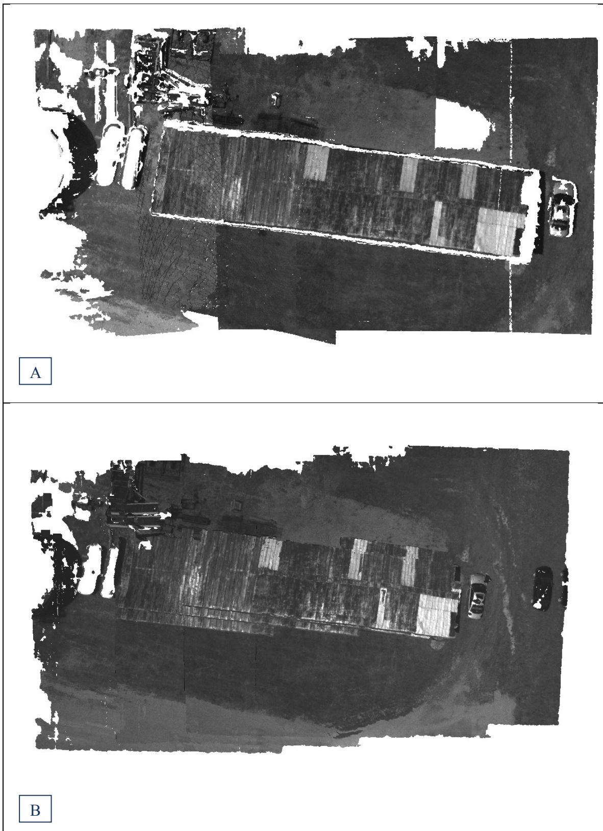
Figure 5-12. 3D reconstructed model of the shed in April 14 dataset using local dense bundling (A) and raw, uncorrected SGBM (B).
