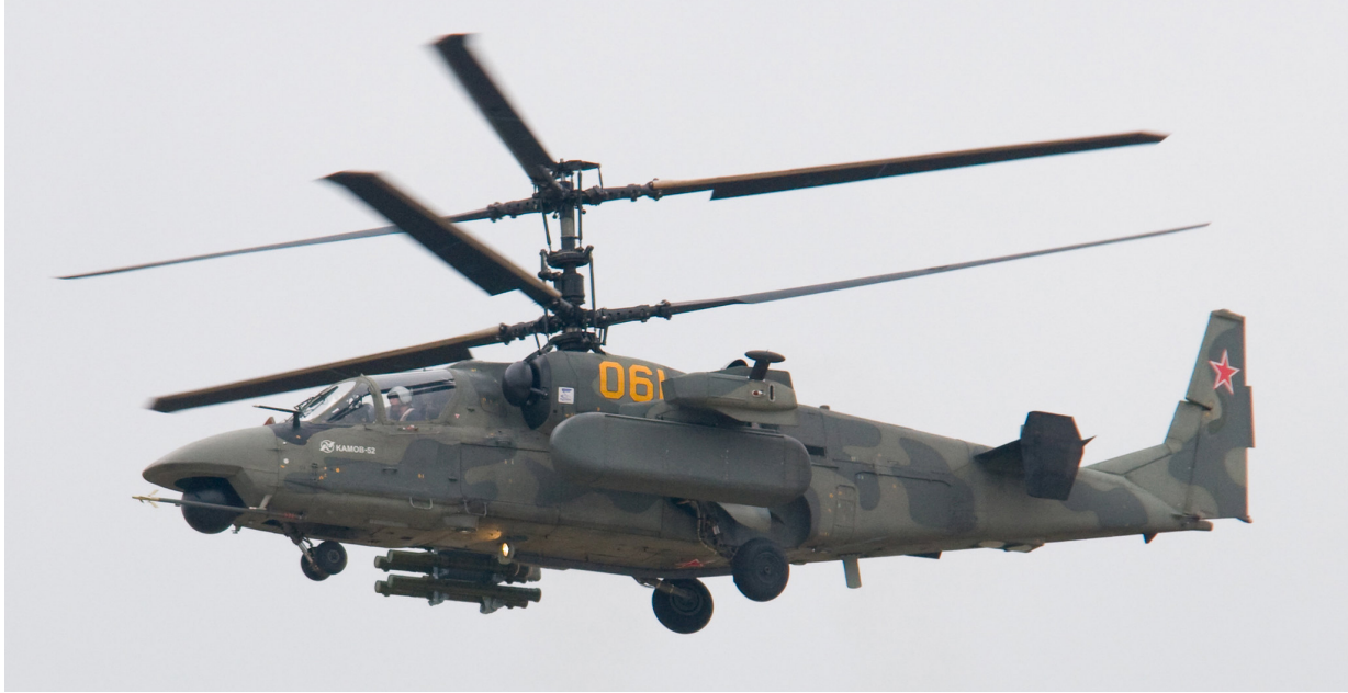
Figure 4.11. [45] Russian Airforce Kamov-52 attack helicopter. Rotorcraft such as this are often favored for the superior safety of the coaxial rotor design and lack of high frequency vibration, making them ideal for targeting systems on military aircraft [37].
