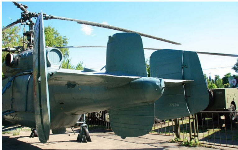
Figure 5.4. [1] Control surfaces on the Kamov Ka-25 coaxial dual-rotor attack helicopter, assisting with maneuverability at speed at the expense of zero-speed turning agility.
