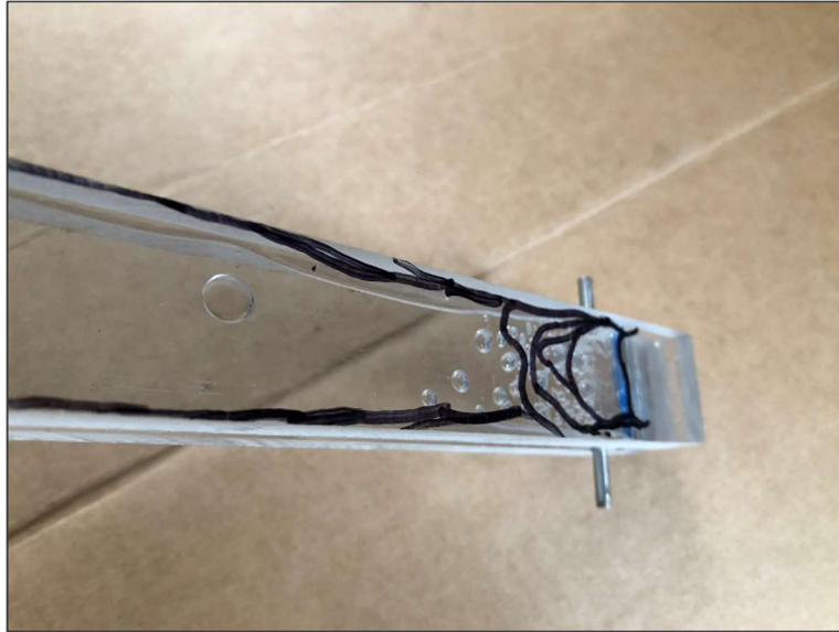
Fig. 30: Extensive cavitation is observed in a wedge test sample with TPU #4. A solitary bubble has formed along the length of the samples far away from the typical cavitation observed for the wedge tests that forms in a cluster close to the wedge.
