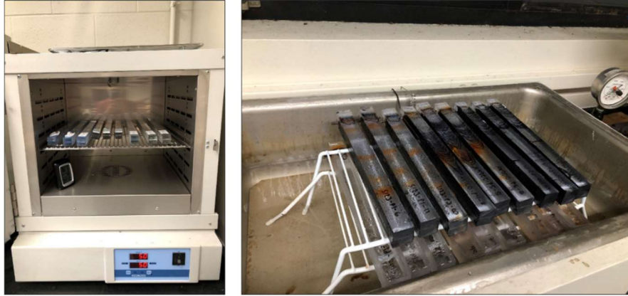
Fig. 6: Dry wedge test samples held in oven at ambient laboratory conditions (left); Wet wedge test samples held suspended in water bath (right)
