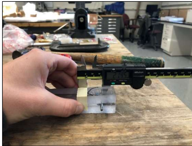
Fig. 7: Measurement of crack length from wedge tip to farthest extent of cavitation/debonding
