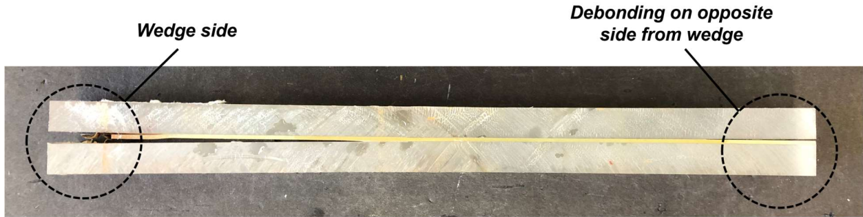
Fig. 17: (EVA 75°C wet) In some of the wedge test samples, the adherends on the side of the sample opposite the wedge began to separate.
