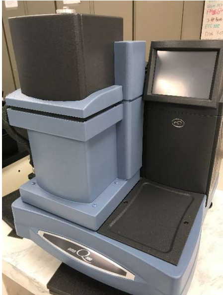
Fig. 9: TA-Q800 DMA machine used for DMA testing to characterize viscoelastic properties of TPU films.
