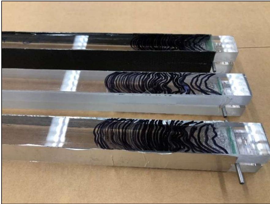
Fig. 8: Wedge samples provided by JNI Armor with edge seals already applied.
