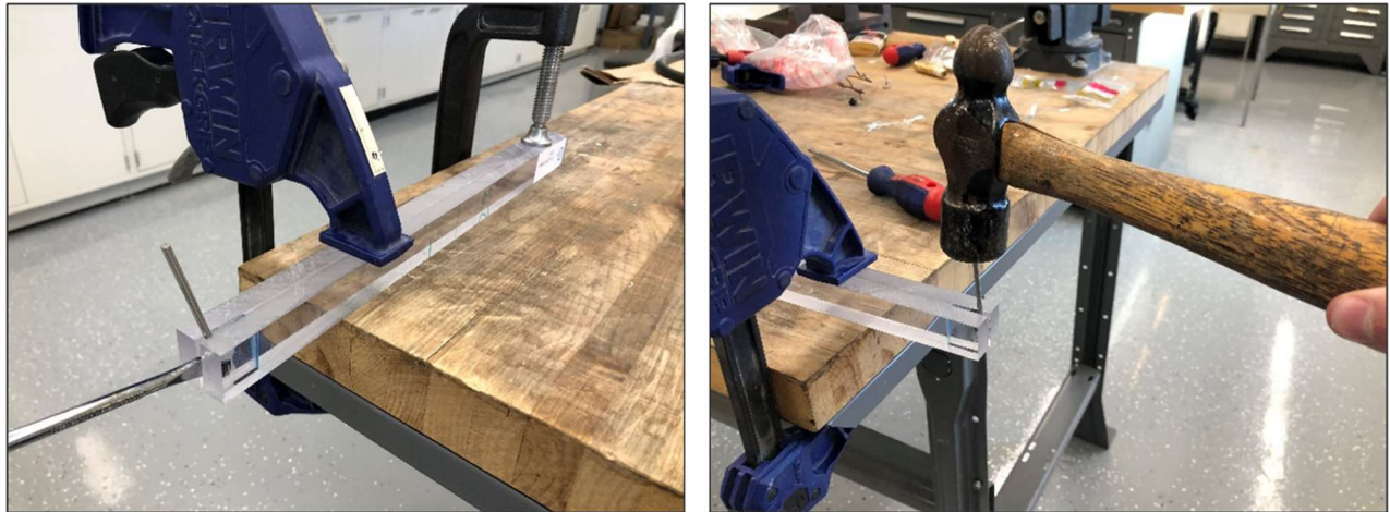
Fig. 5: Insertion of dowel pin into wedge test samples
