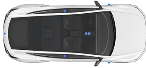
Figure 1.2: 8 cameras on Tesla Model Y [2]
