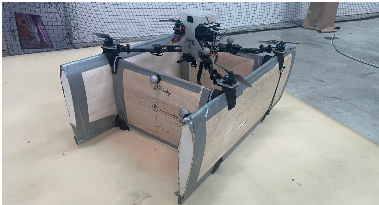
Figure 3.1: The Quad-Rotor Biplane with Vicon-Motion Capture reflectors as used with indoor flight tests.
