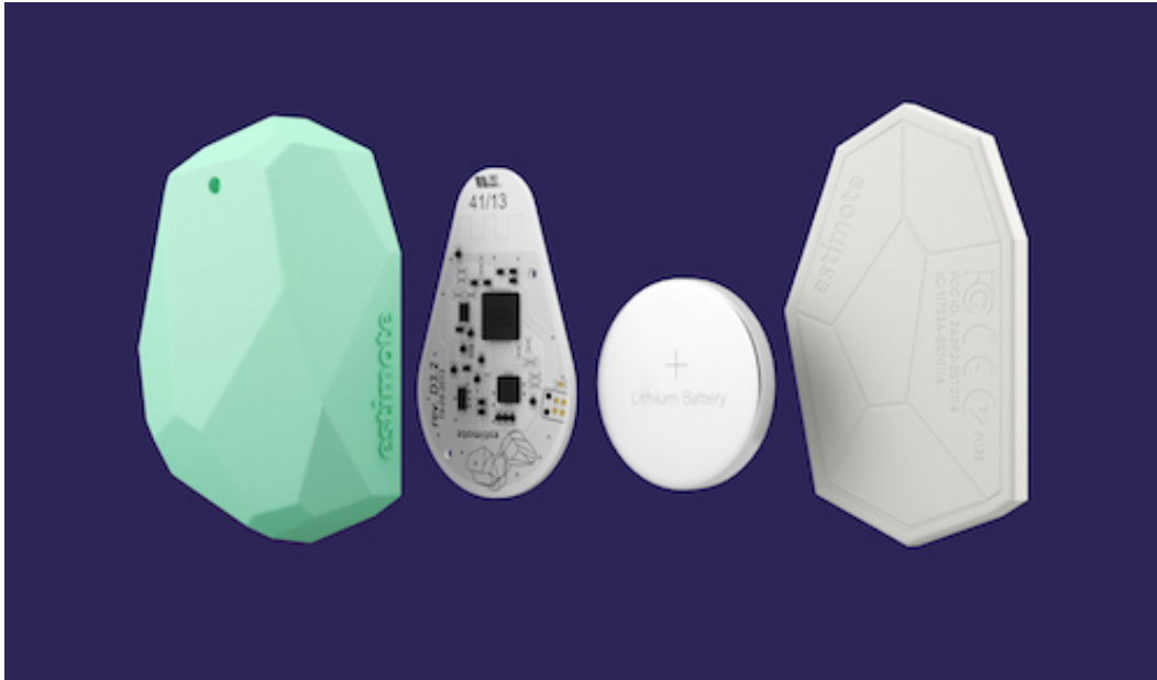
Figure 13. A cross-section of the newer revision of Estimote beacons, showing the battery location. Photo courtesy of Estimote, Inc.
