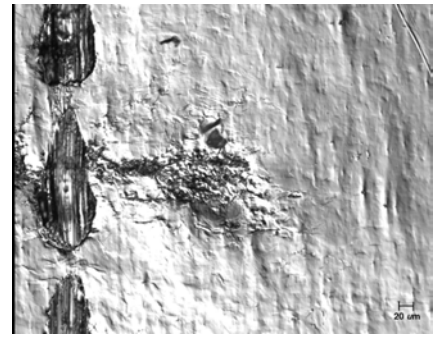
A36, before overload 4, topo
