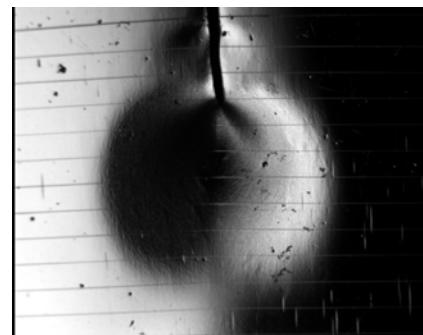
A588, after overload 11, topo
