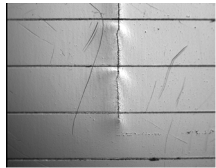
A514, before overload 7, topo
