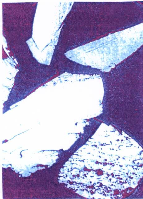
Photograph A. Filter Media with \text{MnO}_x(\text{s}) Coating.
