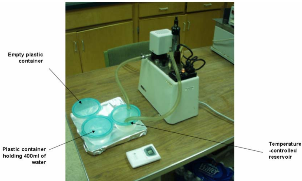
Figure 5.6. Bioassay arena used in the bioassay to determine the effect of thermal shadows on termite aggregation.
