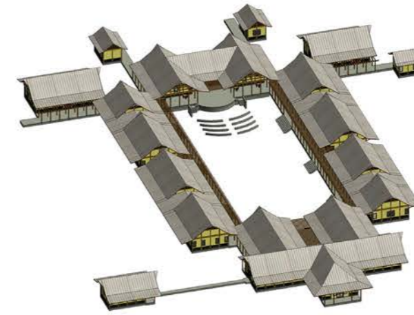
Phase 11: Install pergola members, install site components, install interior walls, install electrical and plumbing, and move in furnishings
