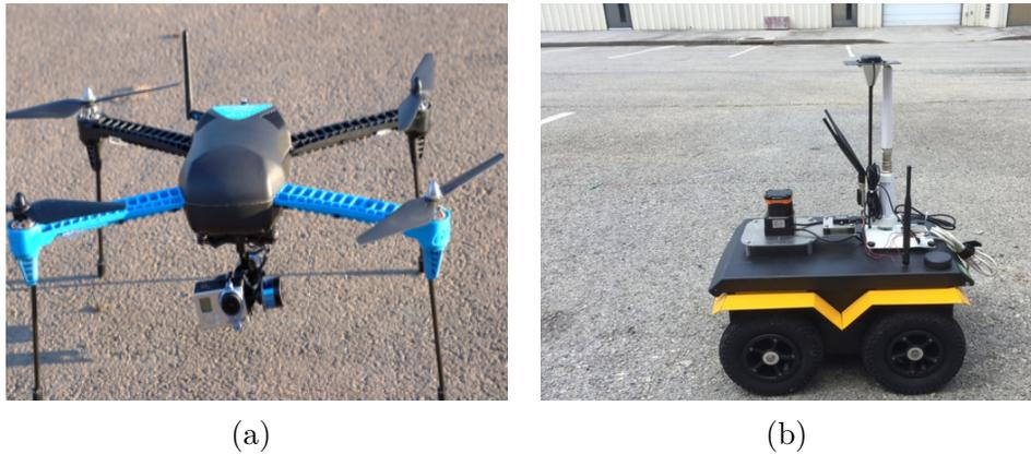
Figure 5.3: Images of data collection hardware: (a) Image of unmanned aerial vehicle (UAV), 3DR Iris quadrotor, on ground before takeoff [52]. (b) Image of unmanned ground vehicle, Jackal by Clearpath robotics.
