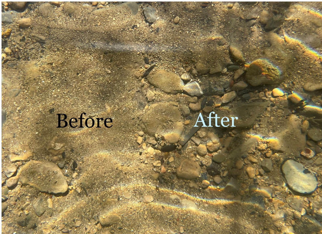
Figure 2.3: Stream bed fine sediment presence before and after an erosive test was performed to determine entrainment with the Benthic Cannon
