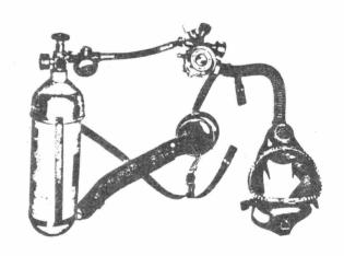
difficult to get the air tanks refilled. Depending upon the size of the tank, the air supply will last up to an hour. There is usually a warning bell that can be set to warn the fumigator when his air supply is running low. The disadvantage of the air pack is that the fumigator has to carry a heavy tank while he completes his work. Already-purchased Bureau of Mines approved self-contained breathing apparatus will be approved for use until March 31, 1979.
