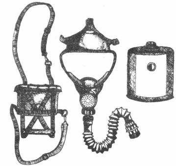
of date used, length of time, and gas concentration should be kept. When a canister is no longer useful, or is being discarded because of use, destroy or mutilate the top so that no one else can use it.
