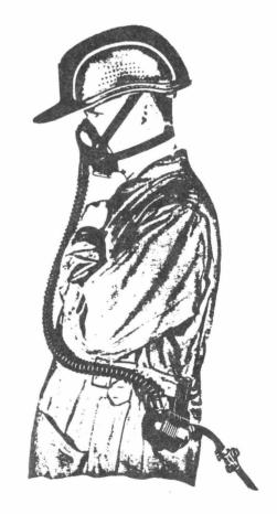
off the air supply. The engine may fail. The air-pump must be located so that contaminated air is not pumped to the fumigator. Care should be taken to avoid cutting or damaging the hose. Already-purchased Bureau of Mines approved air respirators will be approved for use until March 31, 1980.
