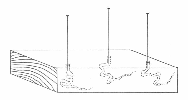
Powder-post Beetle Emergence Holes In Wood NOTE: pins perpendicular to wood surface and shallow penetration
