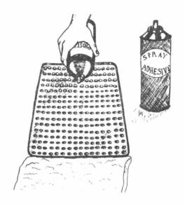
in making sure all edges of the trays are secured. The Phostray or group of trays should then be attached to the top of the load or inside the door used for loading.
