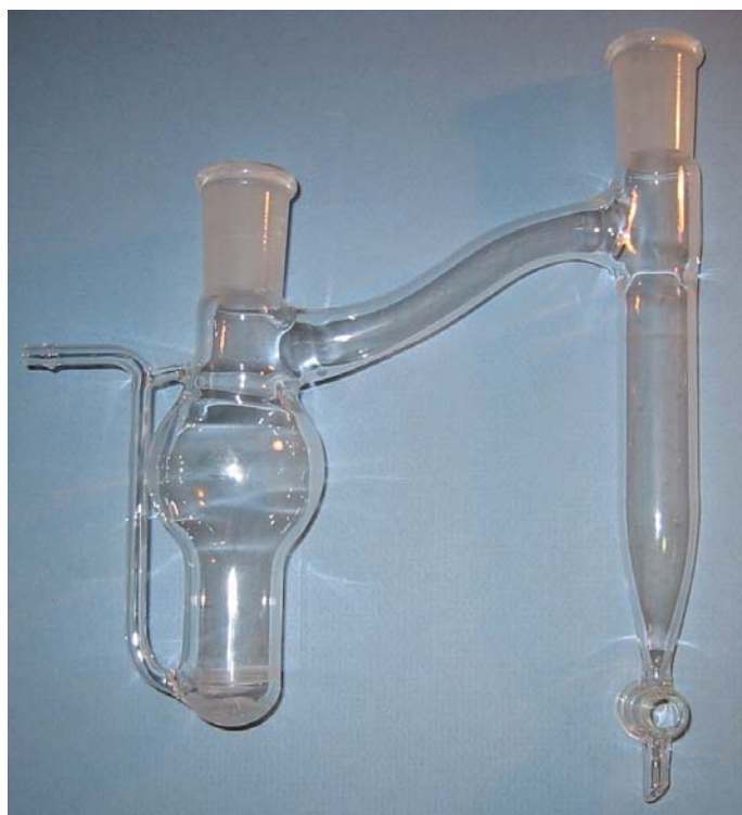
Figure 3.1. Dean Stark Apparatus for Preparing Tetramethylammonium Disiloxanolate Catalyst
