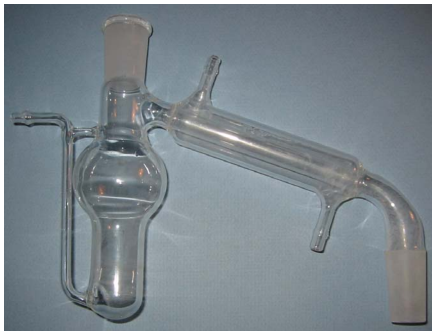
Figure 3.2. Modified Dean Stark Catalyst Apparatus
