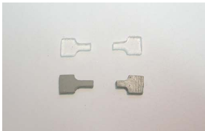
Figure 6.15. Network Tensile Specimens Prepared with a Polyorganosiloxane Substituted with 9 Mol % Nitrile and the Corresponding Thermally Conductive Microcomposite Filled with 67 Volume % Silica-Coated AlN
