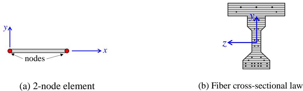
Figure 3.13. Beam elements used in analysis
