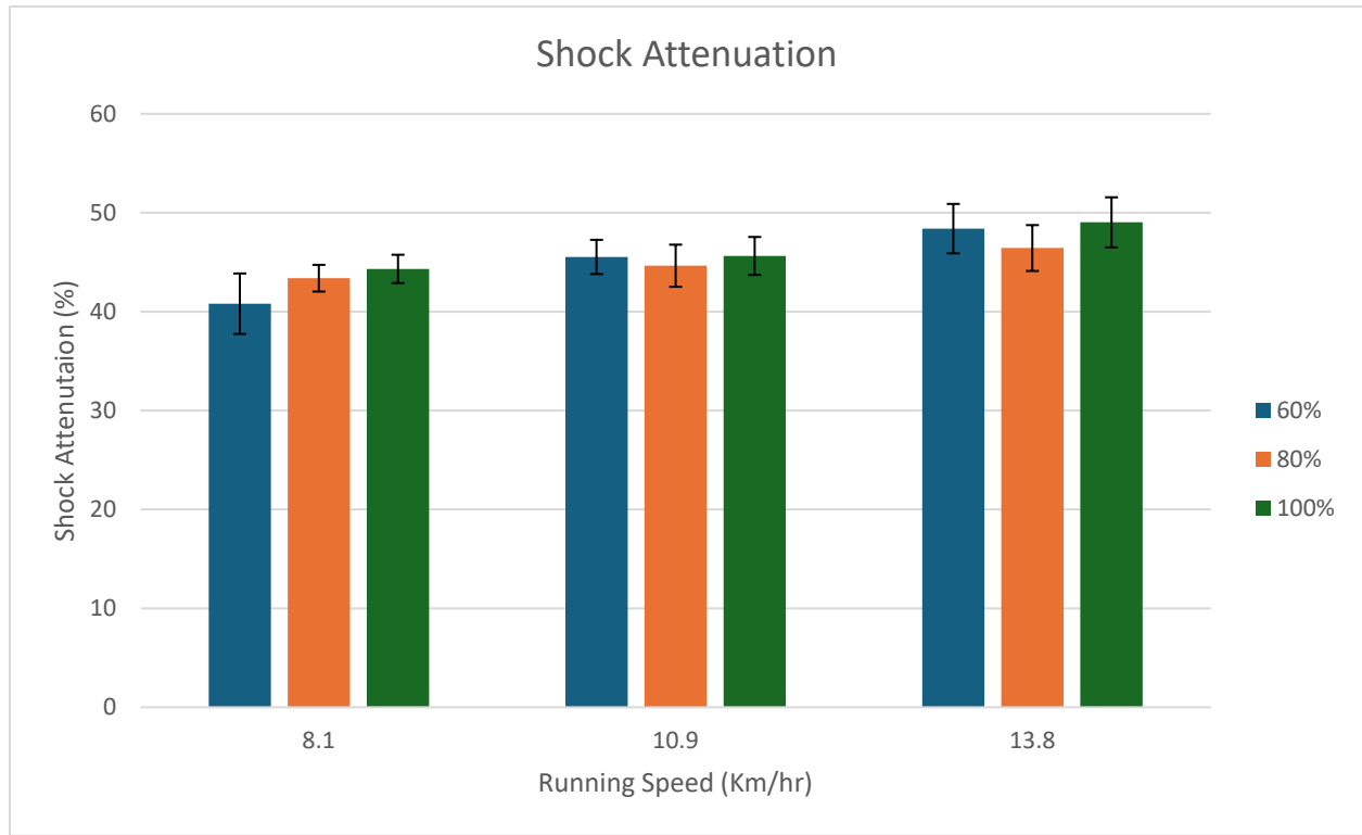
Figure 4.3. Shock attenuation (%) between the tibia and trunk at 3 different running speeds (km/hr) and body weight conditions (60%, 80%, and 100% body weight).
