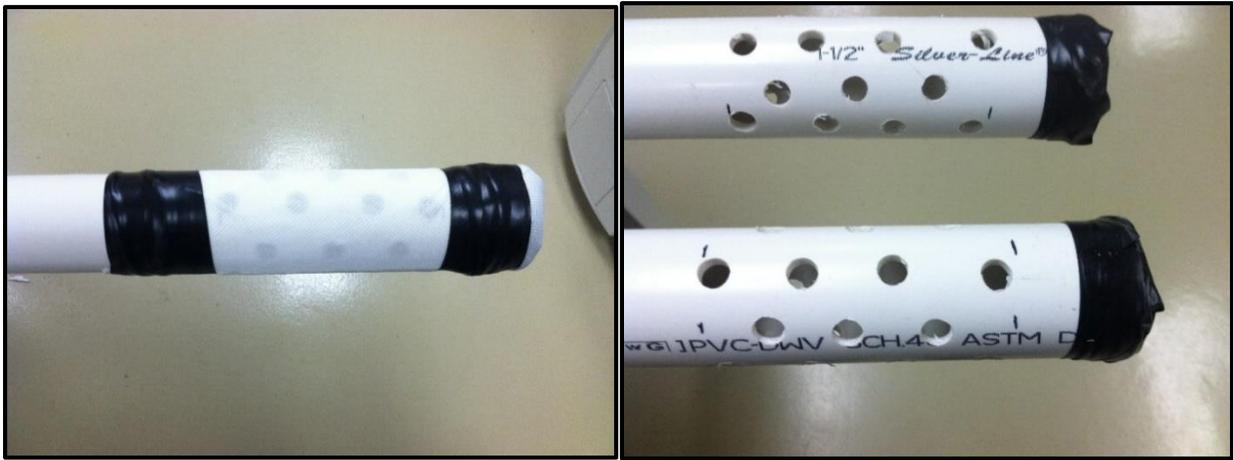
Figure A-2: Piezometer construction method used for all piezometers throughout the site. The screen length was kept constant at 10 cm with the screened interval being between 4 and 14 cm from the piezometer base for each piezometer constructed.
