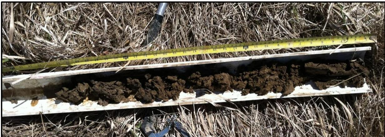
Figure A-3: Example of the method used to visually classify soils during the installation of piezometers 100 cm BGS.
