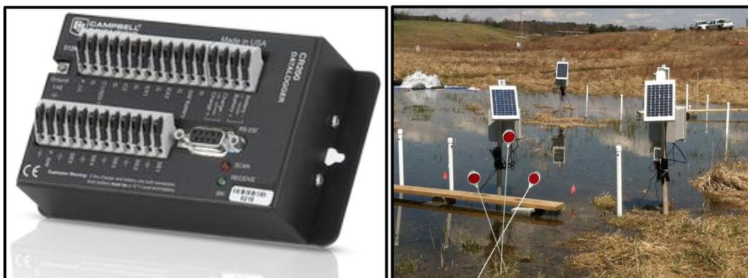
Figure A-5: Campbell Scientific CR200 data logger used for each pair of soil moisture probes (left, [www.campbellsci.com](http://www.campbellsci.com), used under fair use, 2014). The method for housing the data loggers at the site for the entire experiment duration while charging with solar panels (right).
