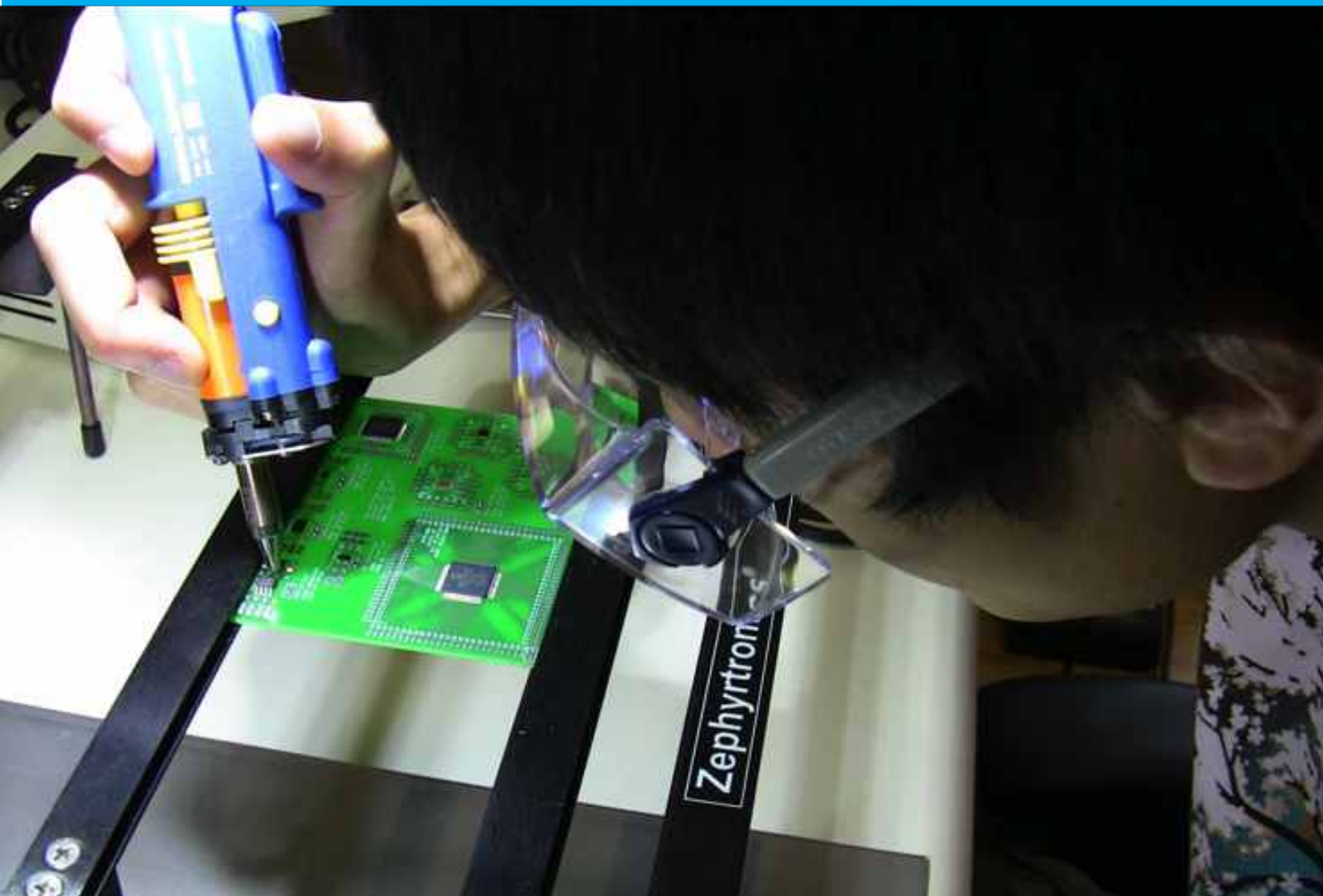
Kevin Lee is removing solder from a surface mount printed circuit board.
