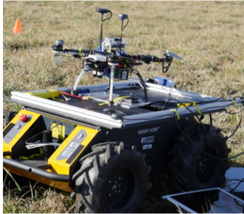
Figure 2.1: DJI F450 with Pixhawk autopilot running APM with onboard Jetson TX1 along with the Clearpath Husky UGV used for the field experiments.
