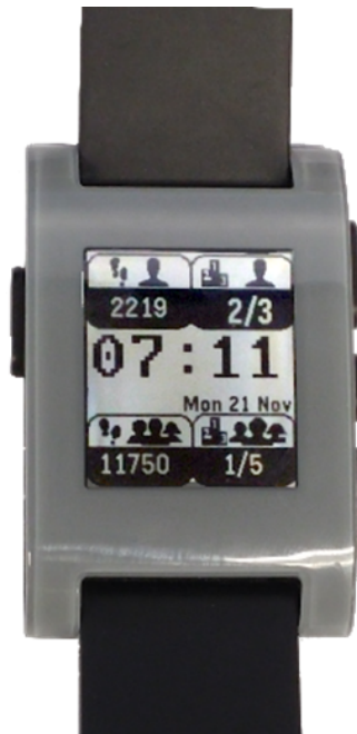
Figure 3.2: The layout of watchface:top left show personal steps, bottom right shows team steps, top right shows user rank in the team, bottom right shows rank of the team among all teams.
