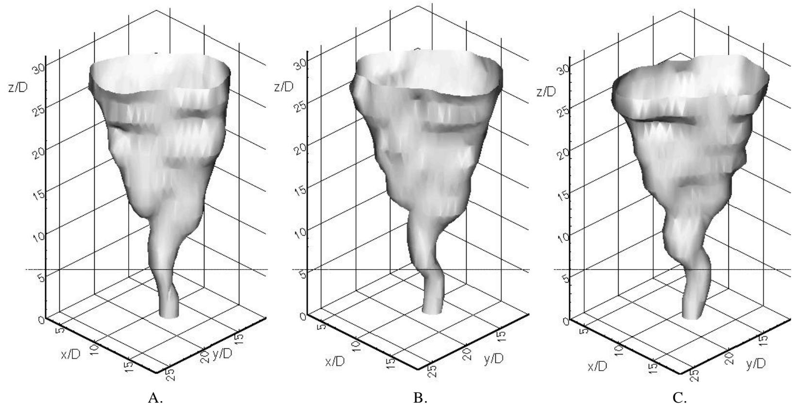
Figure 3.9: 3-D Contours of  $I/I_{\max}(z) = 0.5$  @  $0 \leq z/D \leq 30$ , for a Triangular Jet,  $Re = 8000$ , using Acetone PLIF. A.  $\phi=0^\circ$  B.  $\phi=60^\circ$  C.  $\phi=120^\circ$  D.  $\phi=180^\circ$  E.  $\phi=240^\circ$  F.  $\phi=300^\circ$
