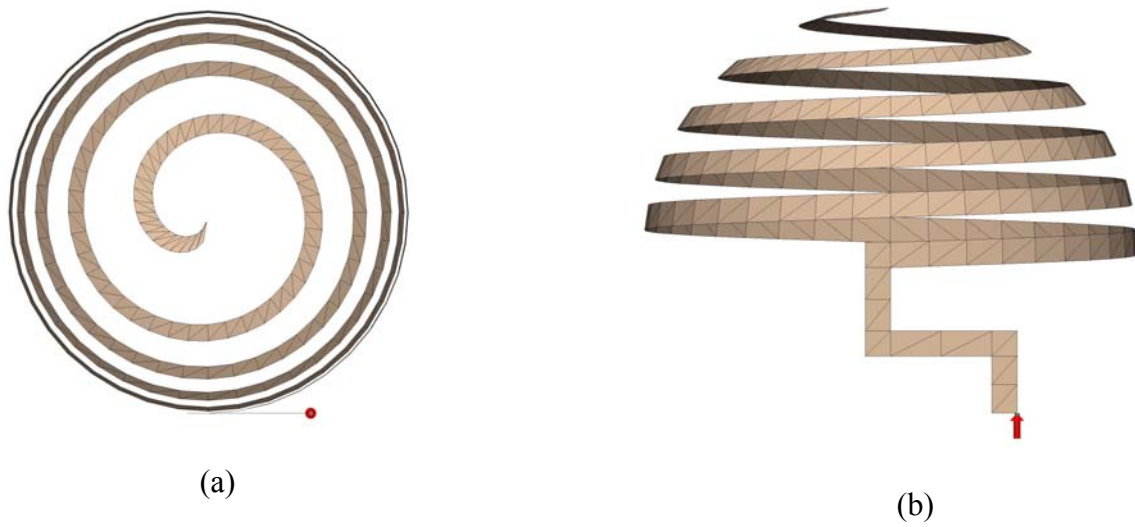
Figure 4.2: Printed hemispherical helical antenna with 2 mm strip width, (a) top view, (b) side view
