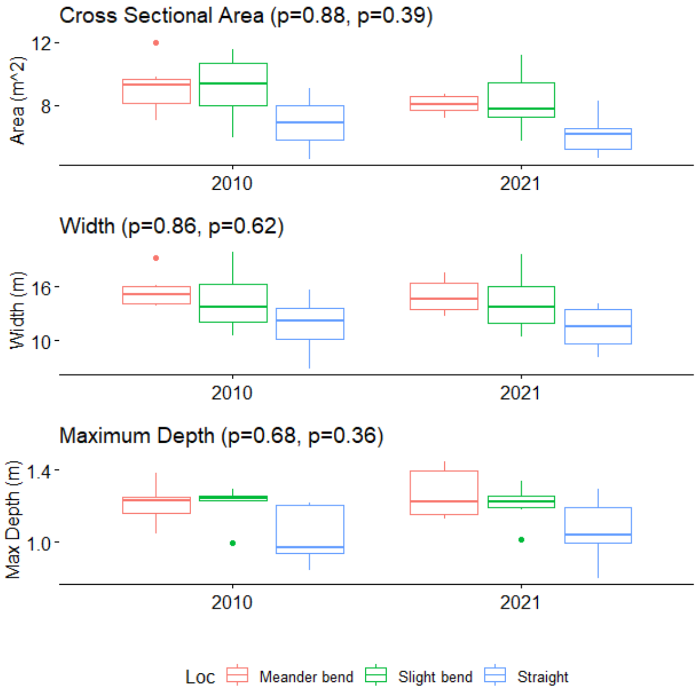
Figure 30: Measured values for area, width, maximum depth, hydraulic depth, and W:D ratio for 2010 and 2021 separated by planform location. Cross Section 5 was removed from the analysis. The first p-value indicates the ANOVA statistical significance of differences in the average percent change among planform locations and the second p-value is the result from the Kruskal-Wallis test. A star next to the p-value indicates statistical significance.
