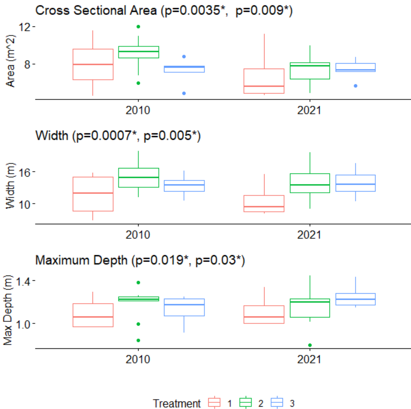
Figure 28: Measured values for area, width, maximum depth, hydraulic depth, and W:D ratio for 2010 and 2021 separated by treatment. Cross Section 5 was removed from the analysis. The first p-value indicates the ANOVA statistical significance of differences in the average percent change among treatments and the second p-value is the result from the Kruskal-Wallis test. A star next to the p-value indicates statistical significance.
