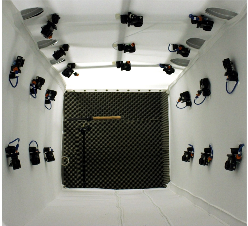
Fig 1. Motion capture system, consisting of 21 GoPro cameras inside a 1.2 x 1.2 meter cross section flight tunnel. The bat was trained to fly through the tunnel and land on the cork perch shown.
