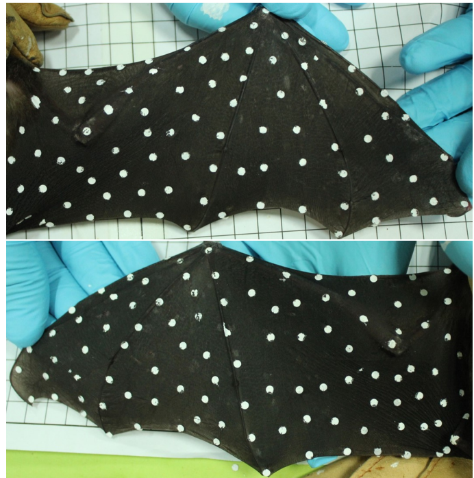
Fig. 8 Several small white landmarks were placed on each bat wing. The number of points defines the spatial resolution of the final data set. Using simple approximations, a lower bound of 70 points should be used, however redundancy makes the data set quality less sensitive to occluded points. Too many points would lead to problems during post-processing, thus the approximately 200 points seen here represents a compromise.
