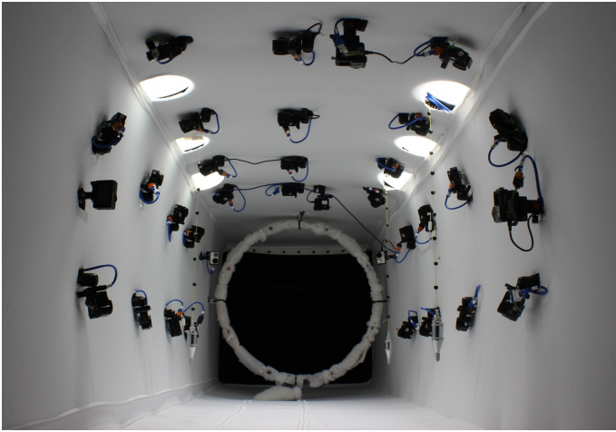
Fig. 2 The flight tunnel was configured for 3D motion capture of bat flight. An array of 34 cameras allowed for redundancy as well as mitigated occlusions of the wing landmarks. Six lights in the ceiling illuminated the subject during recorded to avoid motion blur. Gravity plumb lines establish an accurate gravity vector during post processing.
