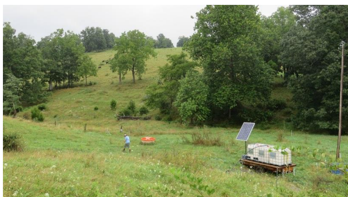
Figure 2. Using solar to pump water from a small spring creek.
