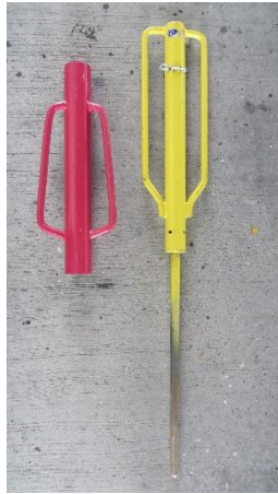
Manual post driver and pilot driver
