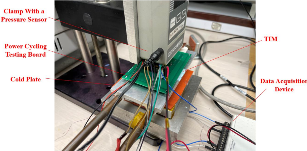
Fig. 4-9. Power cycling setup with a clamp and a water-cooling plate.
