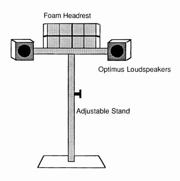
Figure 11. Front view of headrest loudspeaker apparatus.
