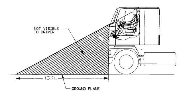
Figure 1. Limited forward ground visibility (from Schmitt 1987).
