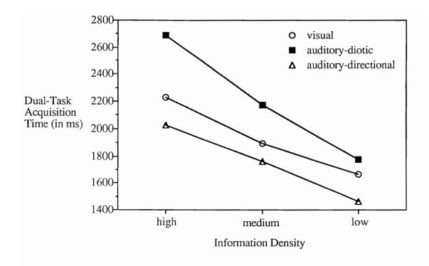
Figure 17. Prompt Type-by-Information Density Interaction for Dual-Task Acquisition
