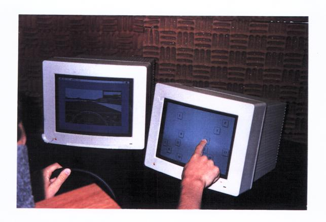
Figure 12. A photograph of a mock participant responding to a prompt by selecting a letter button on the touchscreen during the dual-task scenario.
