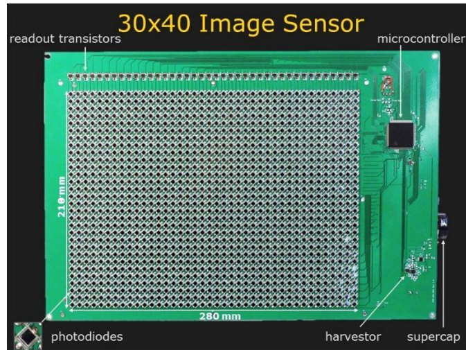
Figure 58. A photodiode array designed to function as a camera (Nayar, et al., 2015). Reprinted with permission, © 2015 IEEE (see Appendix A).
