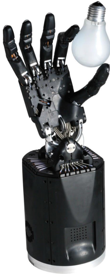
Figure 1. The Shadow Dexterous Hand (Shadow, 2013). Used under fair use, 2016 (see Appendix A).
