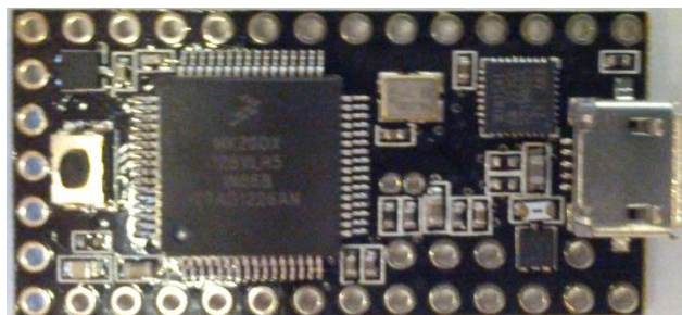
Figure 26. Arduino-based Teensy board measuring 35.5mm in width and 17.8mm in length (Stevens, 2013). Reprinted with permission (see Appendix A).
