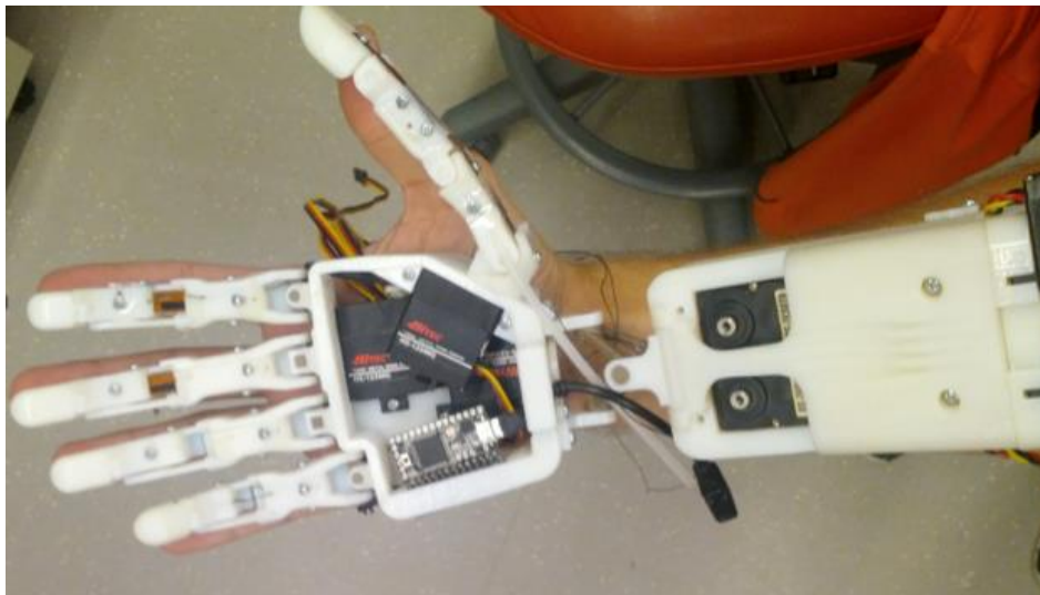
Figure 45. The DASH Hand, shown in comparison with an adult male hand (Stevens, 2013). Reprinted with permission (see Appendix A).
