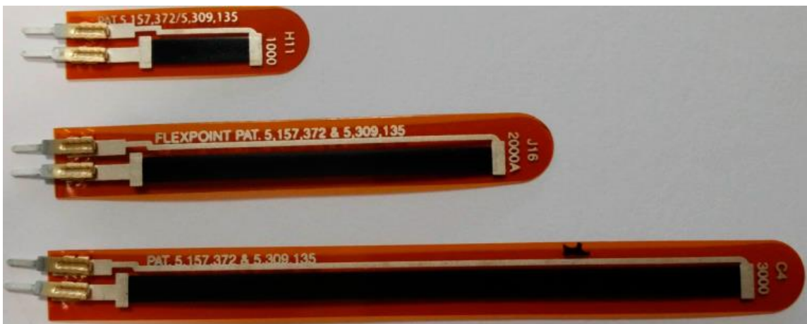
Figure 46. Flexpoint bend sensors, in 1", 2", and 3" lengths (Saggio, et al., 2014). Used under Open Access.
