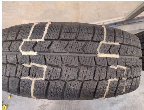
Figure 3-4: Thermocouples fixed in the grooves of the tires
