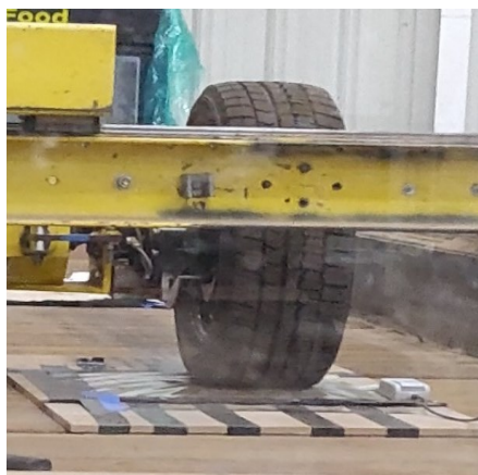
Figure 5-2: Squeezing of the pressure distribution setup when a tire is rotating with 12% slip ratio
