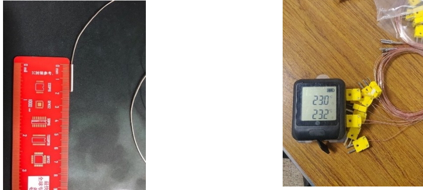
Figure 3-3: K-type thermocouple to attach to the grooves of the tire
