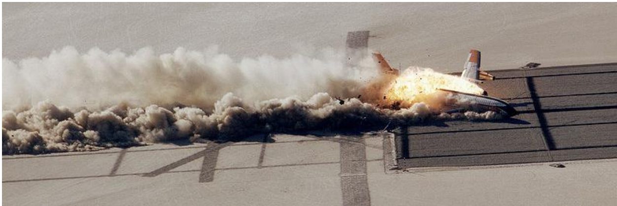
Figure 2.1: Soft soil impact of a Boeing 720 conducted by the FAA and NASA [35].
