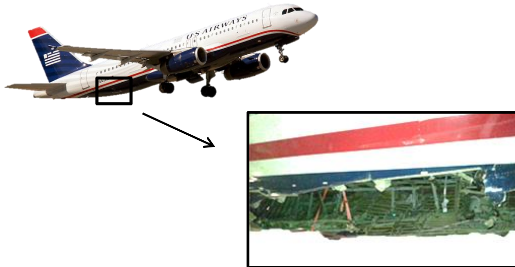
Figure 1.2: Ruptured undercarriage bays of the Airbus A320 that ditched in the Hudson River.
