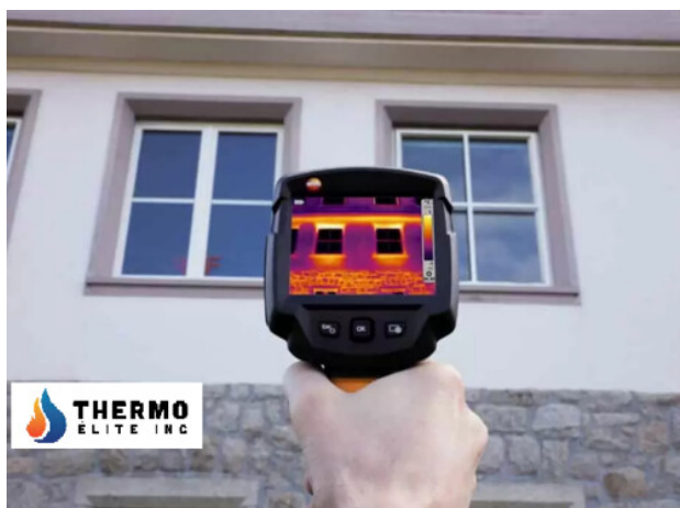
Figure 4.4: Thermographic inspection illustration.
