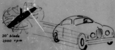
Blade tip speed equals 120 mph.
