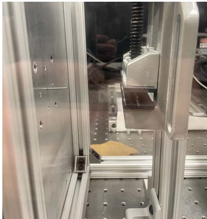
Figure 28: Sample holding vise for sea urchin spine impact tests
