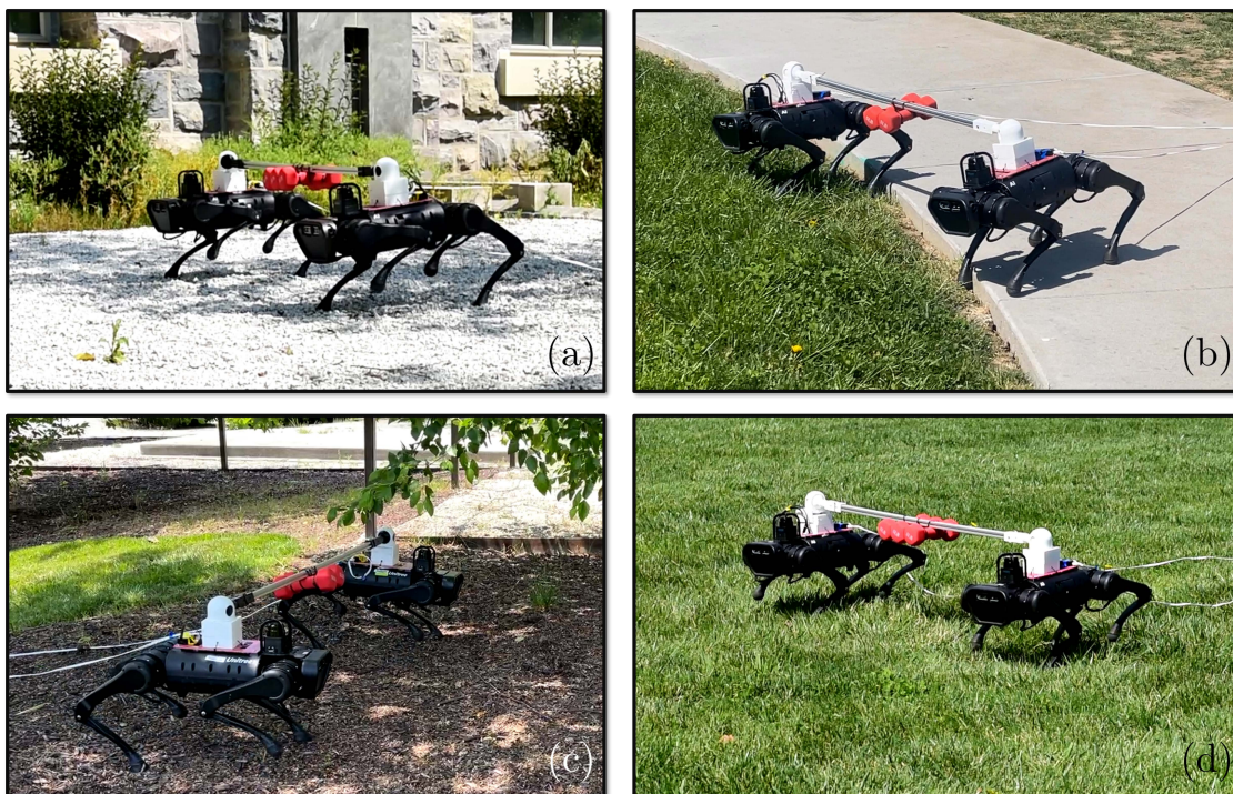
Figure 4.20: Snapshots demonstrate the proposed layered controller’s performance for a series of cooperative locomotion experiments. Outdoor experiments: (a) cooperative locomotion on gravel, (b) transitioning from concrete surface to grass, (c) cooperative locomotion on mulch, and (d) cooperative locomotion on grass. The robots cooperatively transport a payload of 4.53 (kg) (36% uncertainty) in (b) and (c) and 6.80 (kg) (55% uncertainty) in (a) and (d). Here, (a) and (c) show the snapshots where the distributed MPC is adopted, while (b) and (d) show the snapshots where the centralized MPC is employed.
