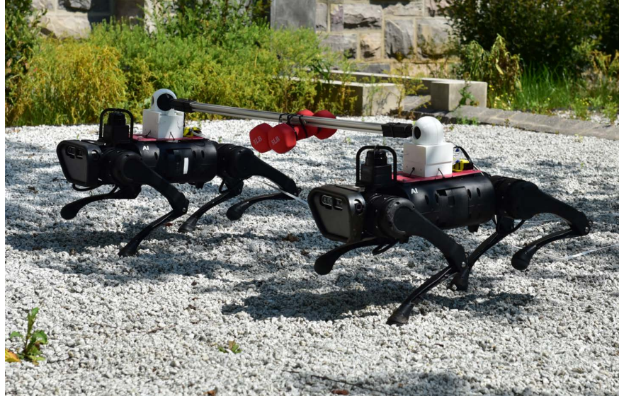
Figure 4.1: Snapshot illustrating holonomically constrained quadrupedal robots locomoting on gravel while carrying a payload of 4.53 (kg).
