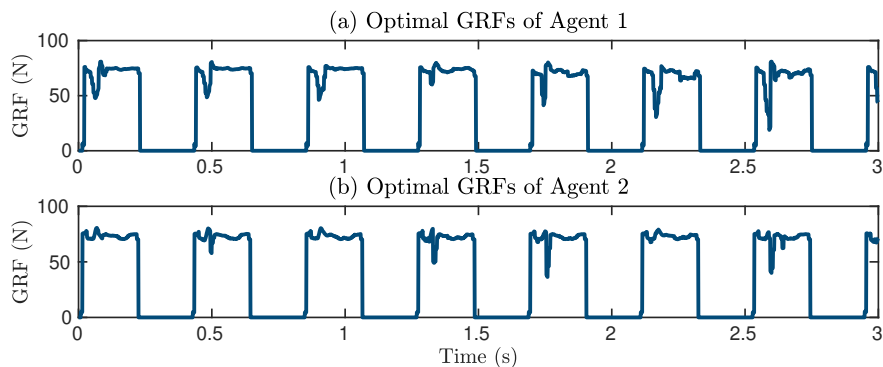
Figure 4.14: Plots of the optimal GRFs generated from the centralized MPC for agents 1 and 2 during the nominal trot experiment on flat ground. The figure depicts the z components of the optimal GRFs for the left front leg of each agent. We remark that the GRFs in the z -direction are close to 60 (N) since the trot gait is adopted and the total mass of the robot is 12.45 (kg).
