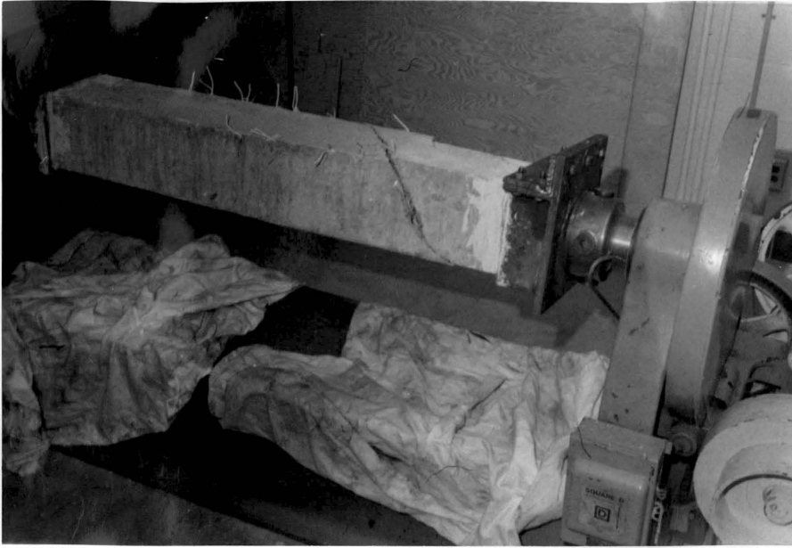
Figure 3-42 Failure Cracks, Beam 2-2
