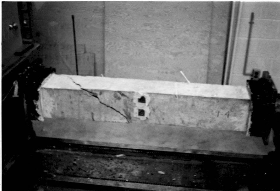
Figure 3-41 Failure Cracks, Beam 1-4
