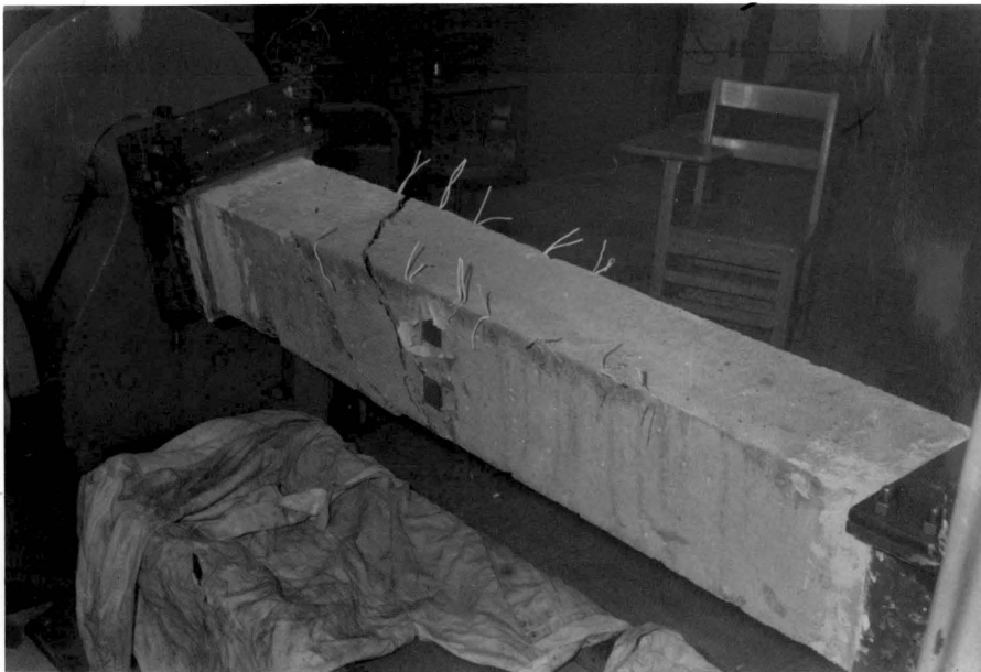
Figure 3-43 Failure Cracks, Beam 2-2
