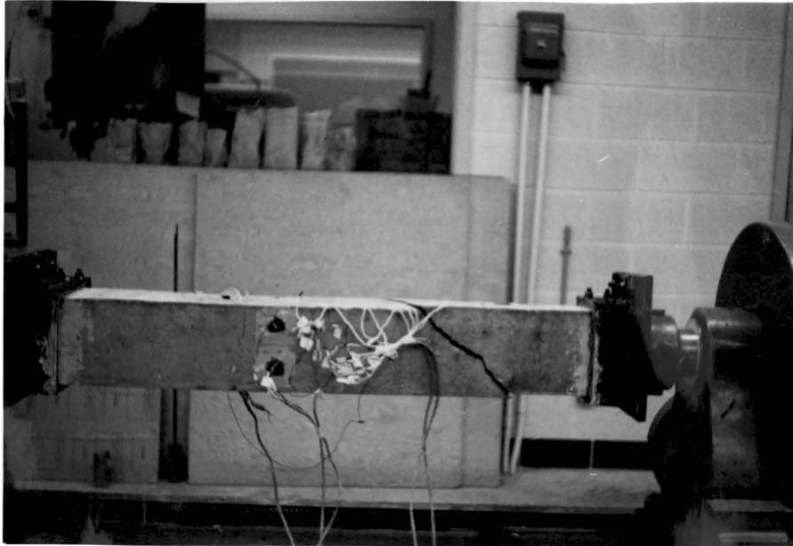
Figure 3-40 Failure Cracks, Beam 1-3
