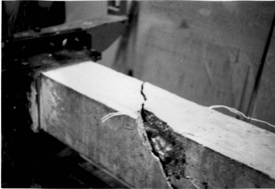
Figure 3-44 Failure Cracks, Beam 2-4
