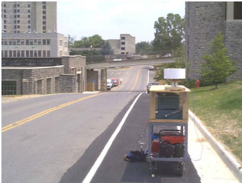
Figure A.2.5: The receiver at location 7 is obstructed by a footbridge. The terrain is hilly and the academic building surrounding this receiver have widely varying heights.
