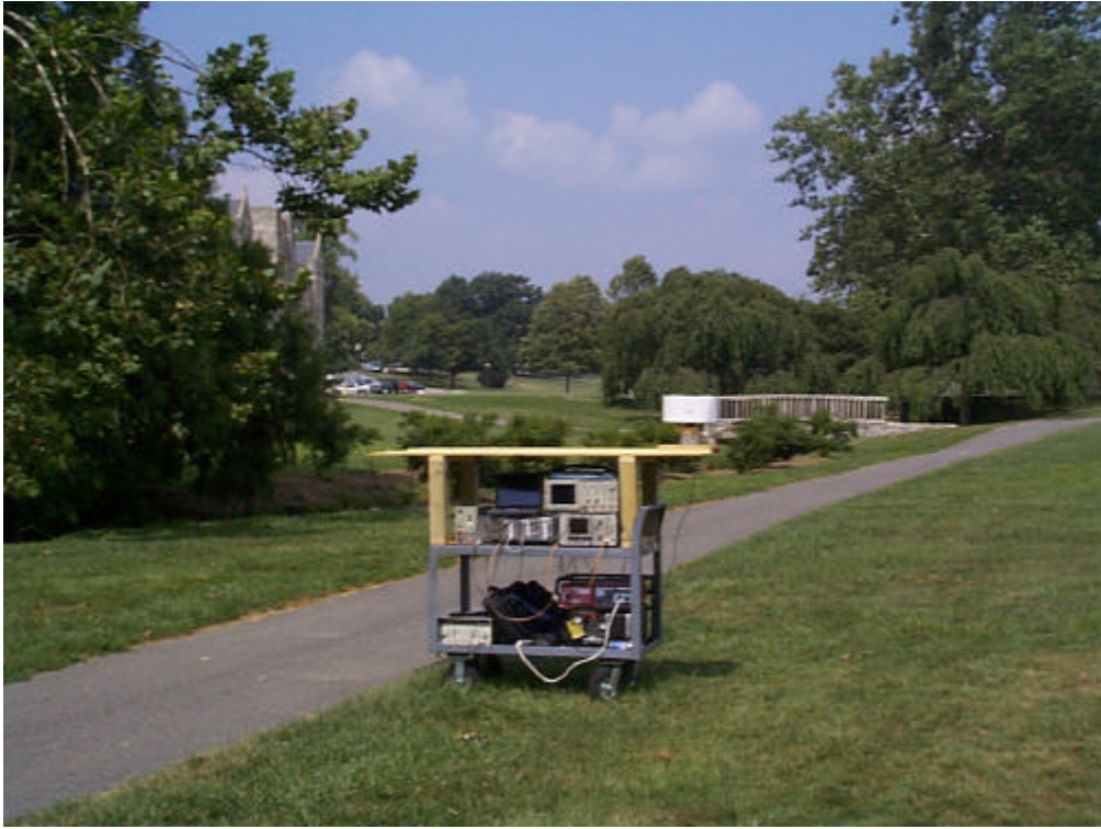
Figure A.4.4: The receiver cart at receiver location 21. The Drillfield is in the background. The link has an unobstructed line-of-sight despite the surrounding trees.
