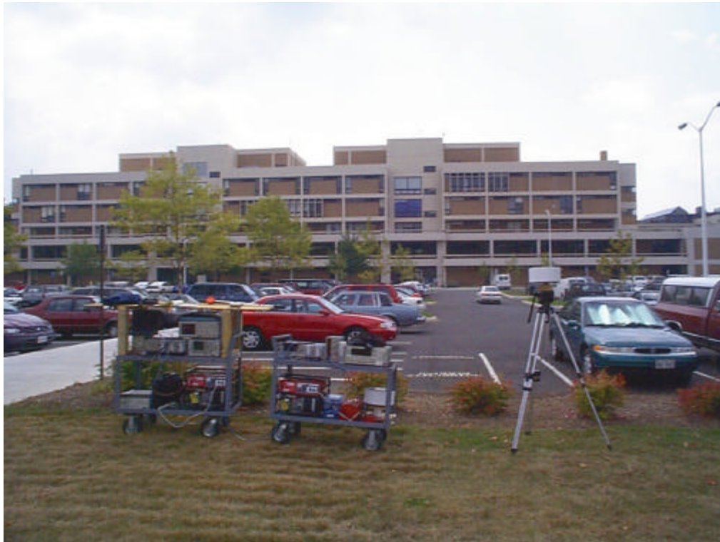
Figure A.3.2: The transmitter location for this site. This photo shows the transmitter and receiver carts connected back-to-back for a calibration test.
