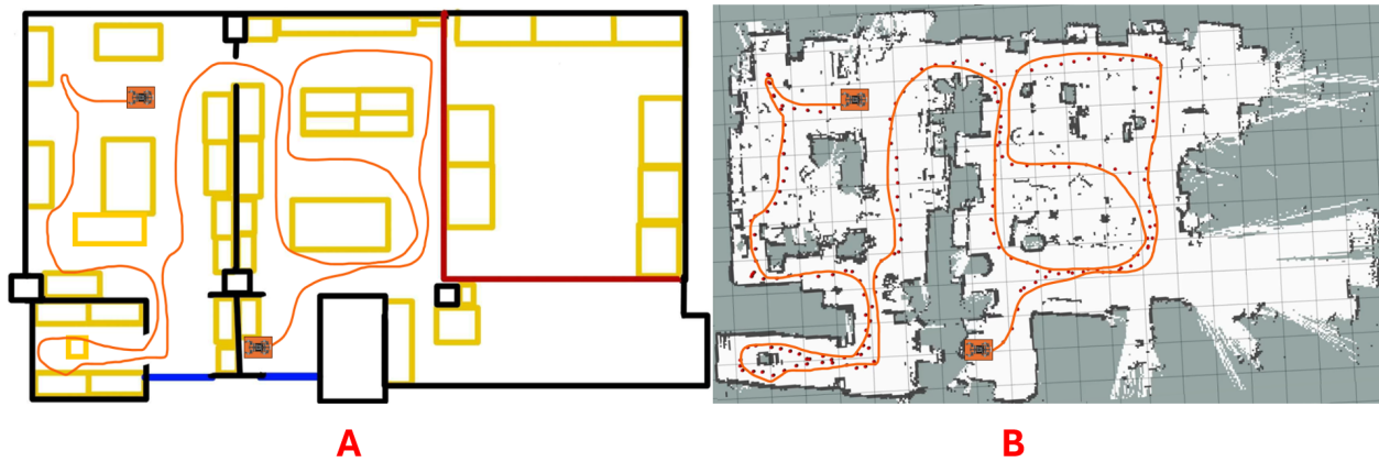
Figure 6.6: Image A shows a simplified building schematic of the lab space with yellow representing approximate furniture placement. The Orange line is Squeaky’s path, which can be compared to the map Squeaky created in Image B.
