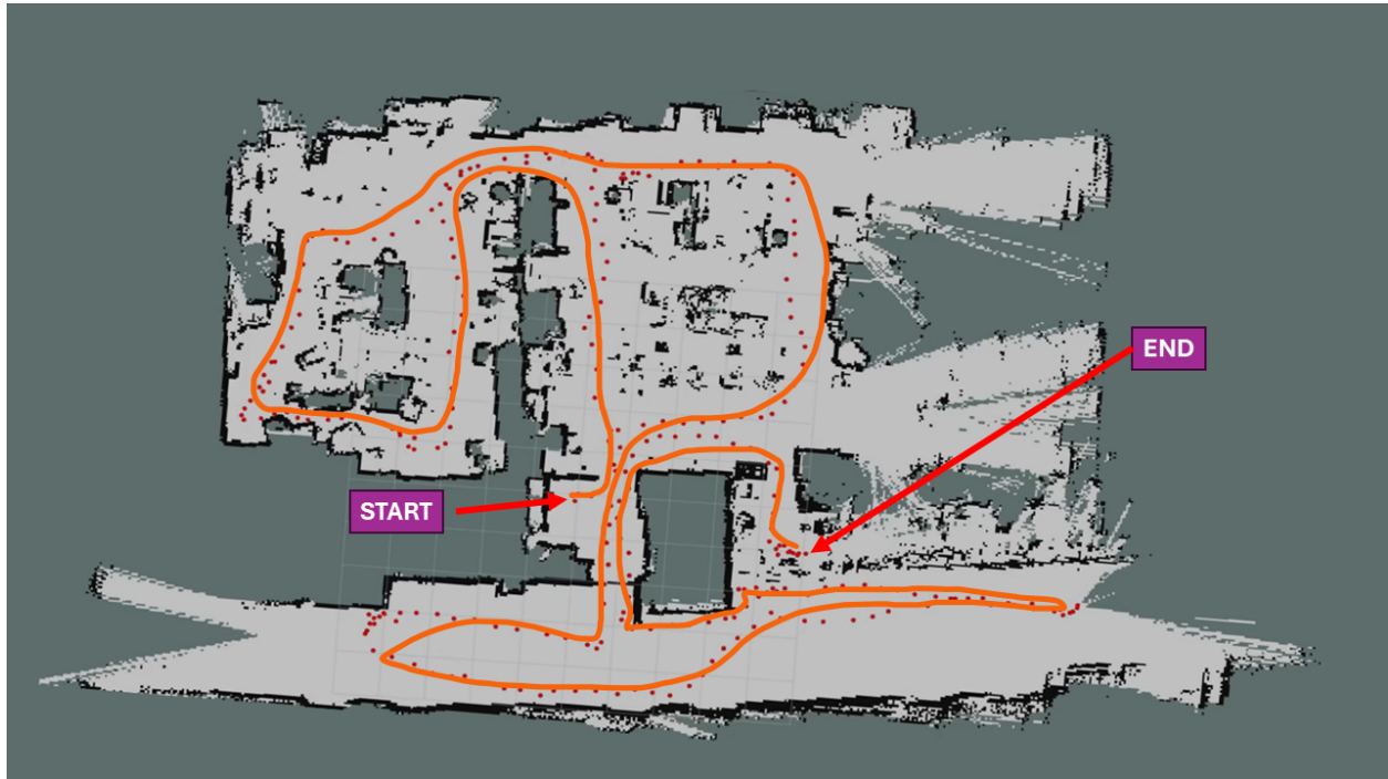
Figure 6.7: Single Squeaky mapping lab space including exterior hallway, 18 minutes to map this area.
