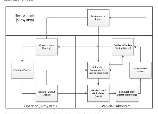
Figure 4-1. Automated Operator-Vehicle Interaction System (Source: Author)
