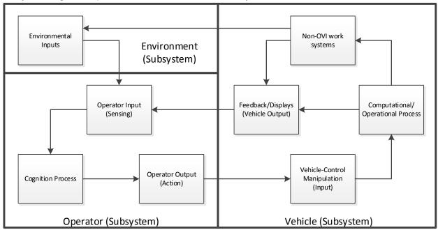
Figure 3-1. Operator-Vehicle Interaction System (Source: Author)
