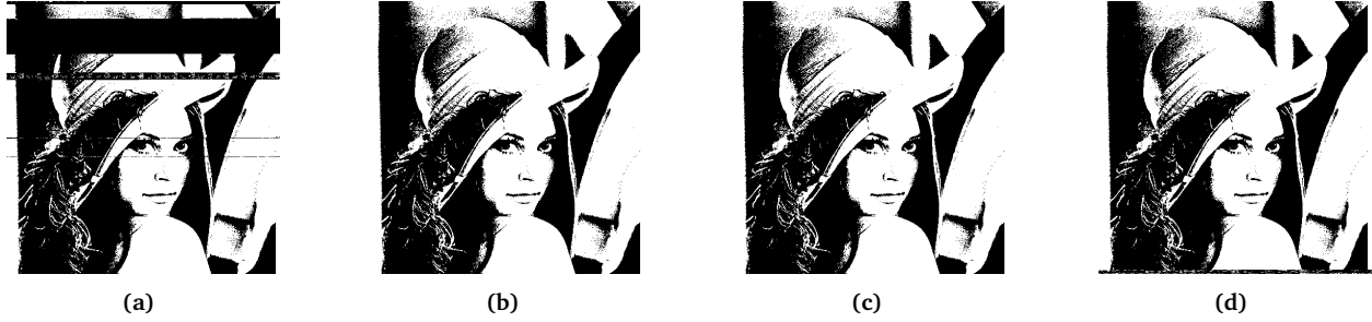
Figure 3.8: Visual representation of iRAM's data extraction for address (a) 0xF8000000 to 0xF8007FFF (b) 0xF8008000 to 0xF800FFFF (c) 0xF8010000 to 0xF8017FFF (d) 0xF8018000 to 0xF8020000 .
