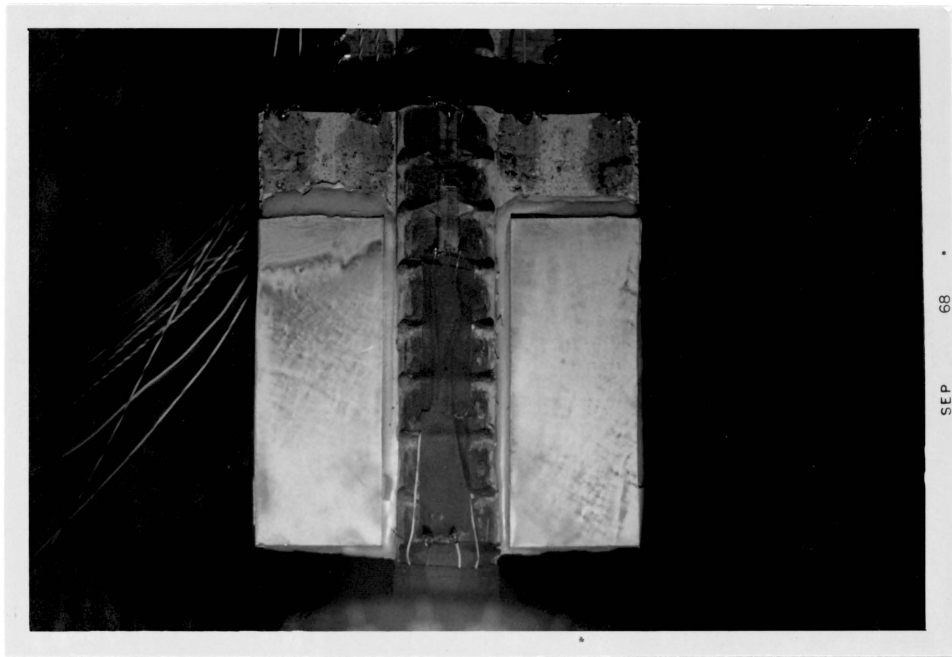
Figure 17. Fringes at Crack Test 3A
