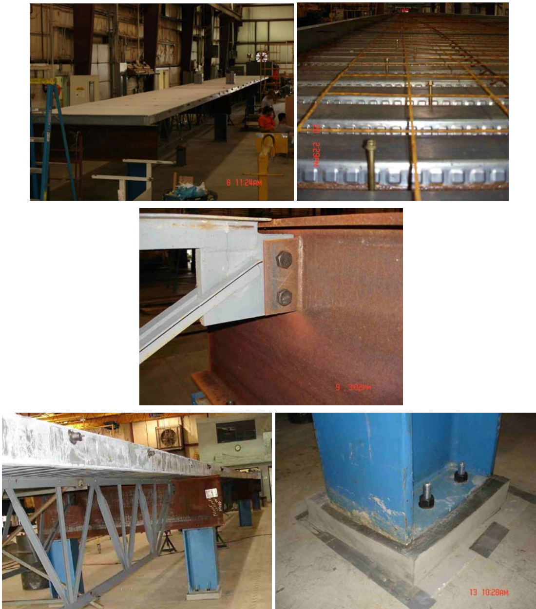
Figure 4.32: Shear Connected Joist Footbridge Pictures
