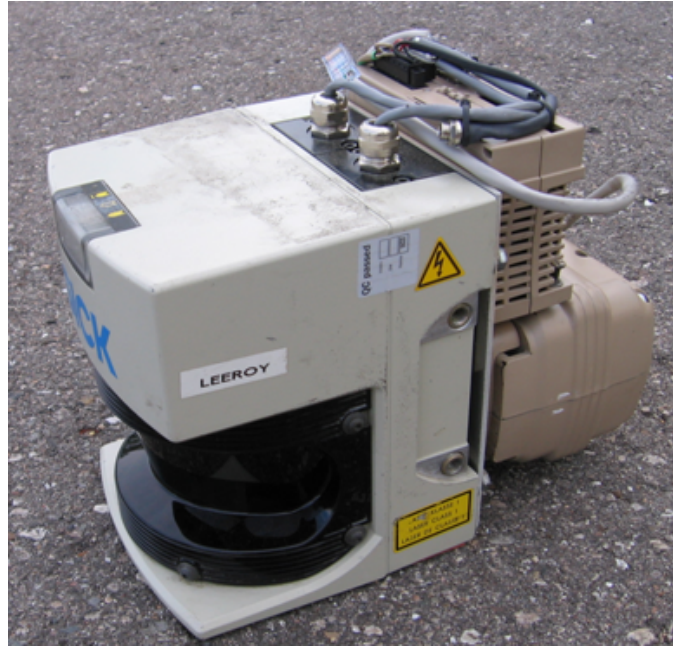
Figure 3.19: Laser Range Finder Payload
