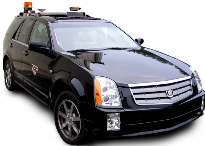
Figure 3.8: Virginia Tech’s JAUS-interoperable Cadillac SRX
