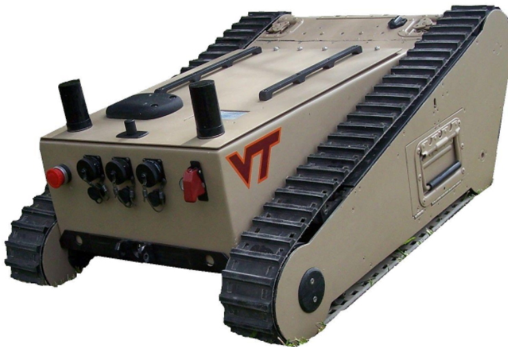
Figure 3.1: Virginia Tech’s JAUS-interoperable MATILDA
