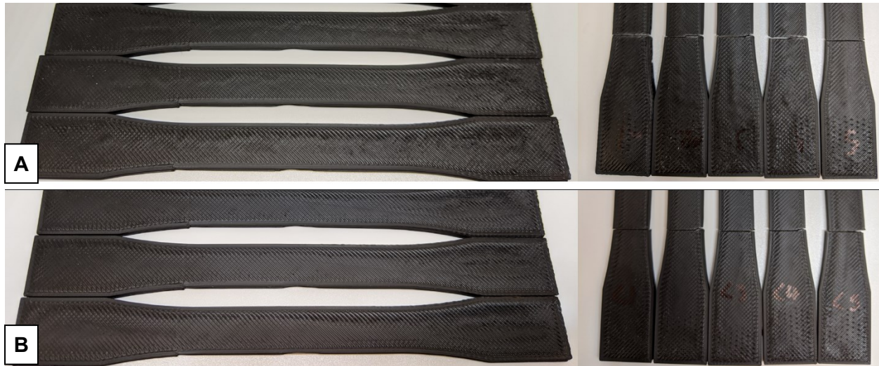
Figure 6.13. Tensile test specimens before and after testing. (A) modulated specimens, (B) control specimens. There is a minor visual difference between the modulated samples and the control samples. This was caused by the modulation creating slightly more roughness on the top surface.
