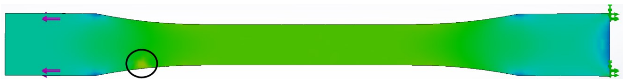
Figure 3.6. Von Mises Stress of a dogbone infected with a void.
