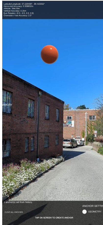
Figure 29. Test of the accuracy of the ball anchor in relation to the longitude and latitude of the Armory
