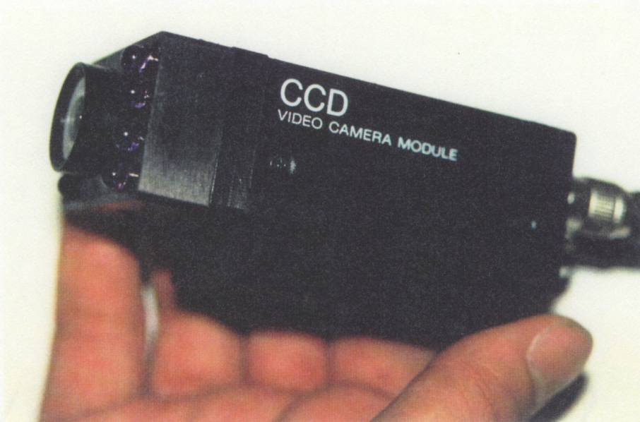
Figure 3.4: Sony CCD Array Camera with LED Light Ring
