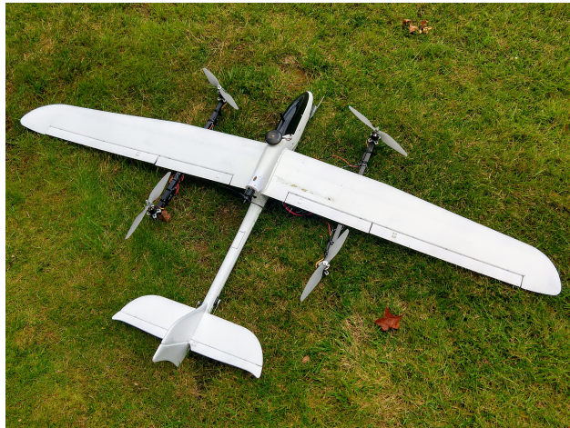
Figure 1.2: Finished Hybrid UAS
