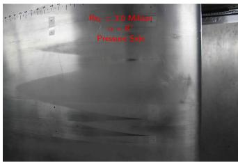
Turbulent wedges caused by tape (40  $\mu$ m) and defects at laminate edges.
