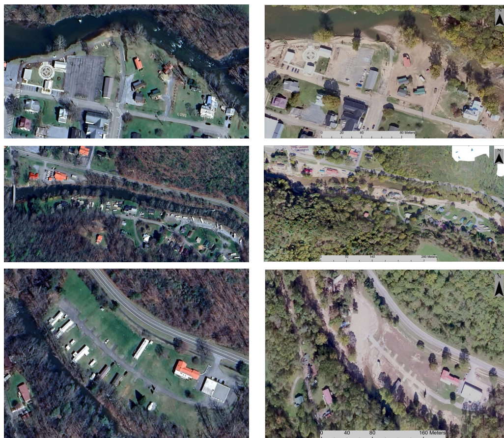
Figure 14. A comparison of pre-hurricane satellite images ( left column ) with post-hurricane ODM orthophotos ( right column ) at three locations (Sections 3, 11, and 10 (top to bottom) from Figure 15) in Damascus. The images on the left are presented at a similar scale to those on the right.
