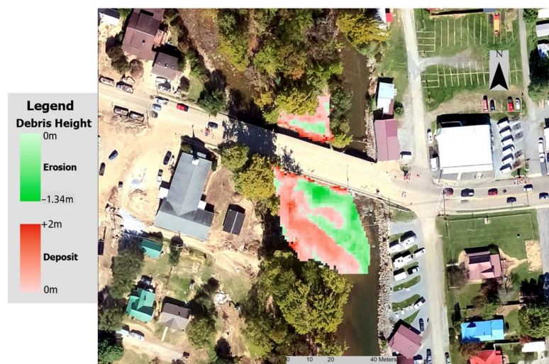
Figure 22. Debris map of a section near the stream, from Figure 16, in Damascus. Here, the green section represents the eroded portion, and the red section represents deposits.
