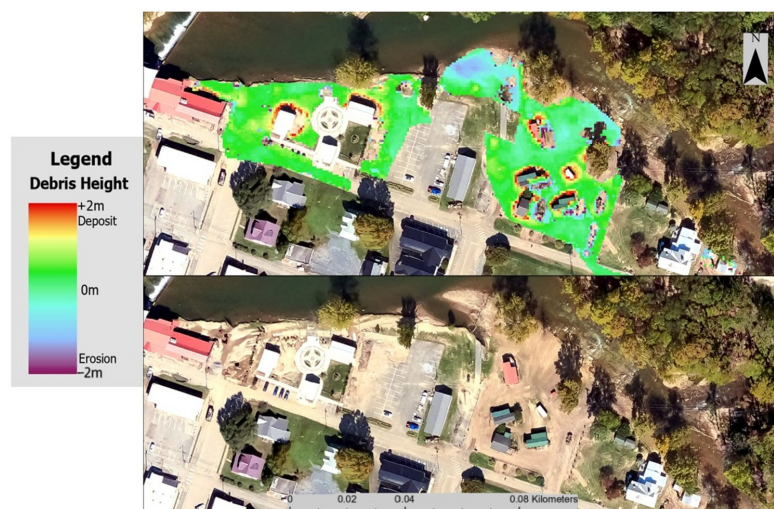
Figure 21. Debris map of sections 3 and 4 of Figure 15 of Damascus. Here, blue represents erosion, red represents high debris, and green and yellow represent moderate debris deposits. (For visual purposes, height differences beyond +2 m and −2 m are omitted for this map, as they are mostly outliers due to misaligned tree and structure heights and shadows).
