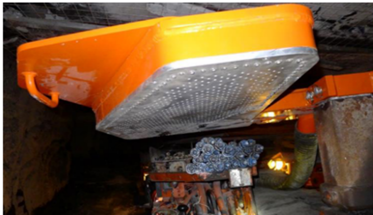
Figure 1.10: A canopy air curtain plenum installed underneath the canopy of a roof bolter to provide filtered air to operators (taken from [8]).
