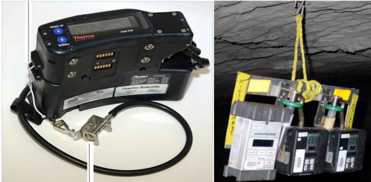
Figure 1.4: The CPDM 3700 sampler (left) and pDR/gravimetric samplers (Right) used for dust sampling and monitoring in coal mines (Taken from [8]).
