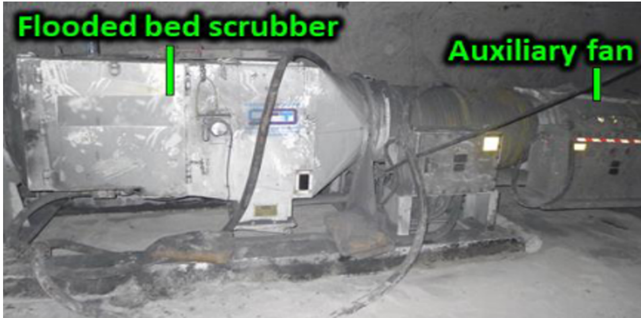
Figure 1.8: A stand-alone flooded bed scrubber used to suppress dust in underground coal mines (taken from [8]).
