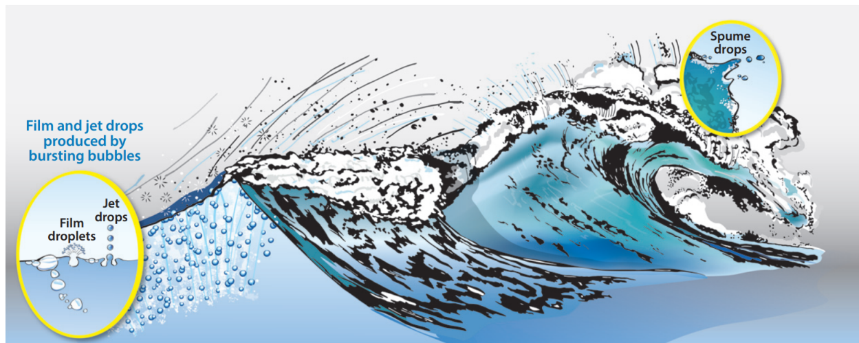
Figure 1.1: Spray aerosol ejection pathways. Ejection pathways of spray aerosols emitted from breaking waves. Adapted from Veron [16].
